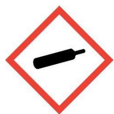
Gas under pressure
