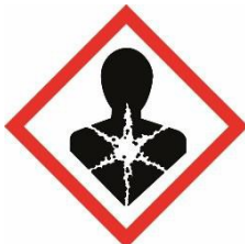
Hazardous to health
